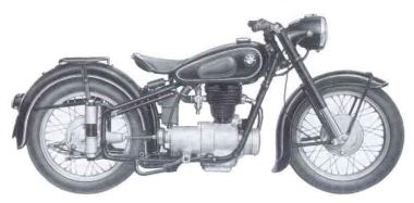
Powerful single cylinder engine. Special air-intake ensuring cool and uniform air supply. Elastic clutch. Four speed gearbox with foot change. Hydraulic damped telescopic front fork.
