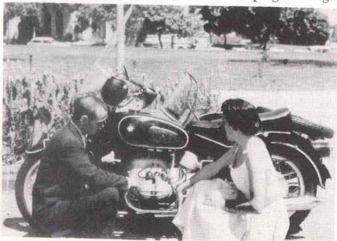
Jim Davis explains to Carol Anderson the details of the horizontally opposed engine of the R69S.
