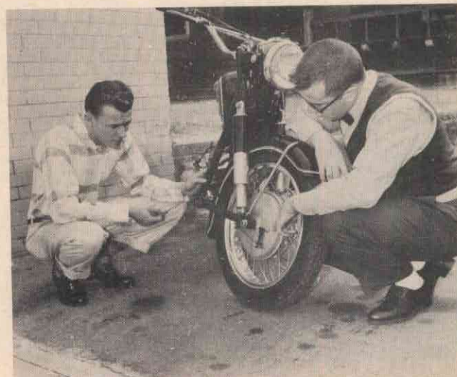
Hot Rod expert, Rick Faucher, showed great interest and approved the front end treatment of the BMW. The Earles fork and the two leading shoes' front brake immediately caught his connoisseur's eye.
